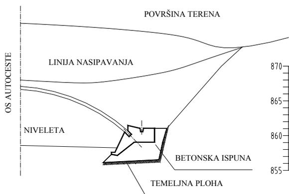
Figure 8. Foundation in the region of clay with rock fragments.
