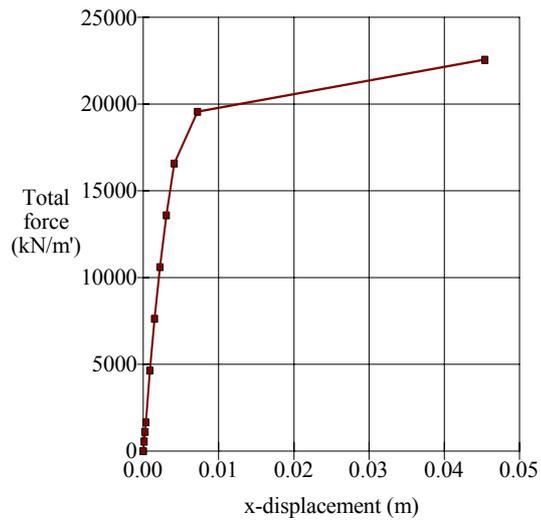
Figure 6. Analysis No. 1: relationship between total force in the arch support and horizontal support displacement.
