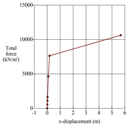
Figure 7. Analysis No. 2: relationship between total force in the arch support and horizontal support displacement (the lower diagram is the enlarged portion of the upper one, up to the value of the design load).
