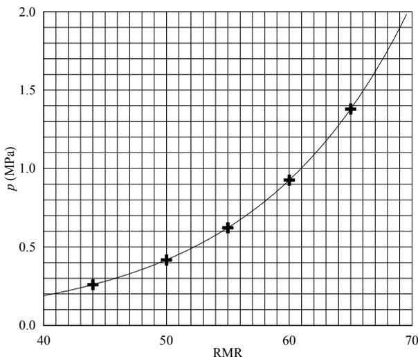
Figure 2. Allowable load  $p$  as a function of RMR for FS = 5.
