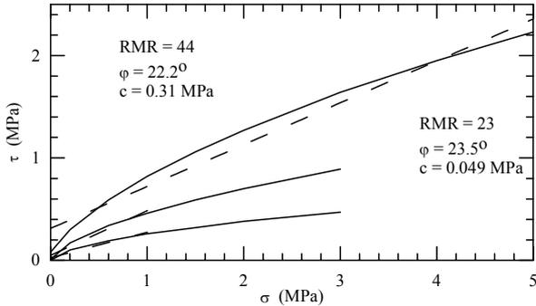
Figure 1. Hoek-Brown strength criterion for RMR = 44 and RMR = 23 and parameters from Table 1 (full line), and equivalent Mohr-Coulomb criterion (dotted line).
